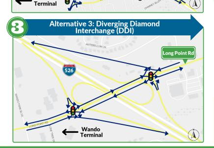
**Alternative 3** would replace the existing interchange with a Diverging Diamond Interchange (DDI). A DDI would remove left turns across oncoming lanes of traffic at each of the intersections within the interchange. This is done by shifting vehicles passing through to the left-hand side of the road. This alternative is compatible with the planned widening of I-526.
