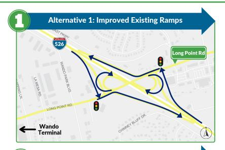
**Alternative 1** would improve the existing ramps. A larger version of the existing interchange, it would address concerns by constructing larger loop ramps to allow for increased speeds to improve merging onto I-526 for all vehicles and be compatible with the planned widening of I-526. Improvements to the eastbound off-ramp would also be made.
